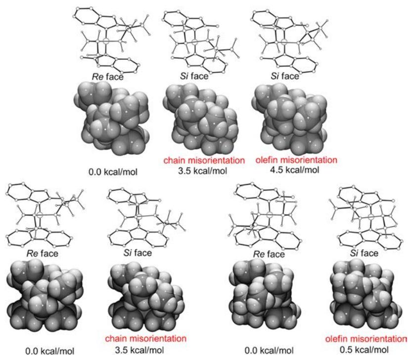
**Figure 58.** Transition states for the  $C_2$ -ansa-zirconocene- and  $C_1$ -ansa-zirconocene-catalyzed polymerization of polypropylene and poly(1-butene). Reprinted with permission from ref 392. Copyright 2007 American Chemical Society.
