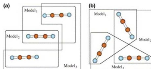
**Figure 15.** Schematic diagrams for the multicentered ONIOM-(QM:QM) approach based on (a) the overlapping and (b) two-body expansion approaches. Reprinted with permission from ref 180b. Copyright 2005 Elsevier B.V.
