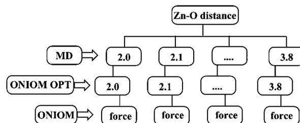
**Figure 13.** A schematic flowchart for the combination of MD and ONIOM methods. Reprinted with permission from ref 172. Copyright 2006 American Chemical Society.
