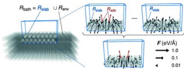
**Figure 9.** A schematic picture in the QM/Me method for metallic systems. The arrows represent computed force ( $F$ ). Reprinted with permission from ref 85. Copyright 2014 Wiley-VCH Verlag GmbH & Co. KGaA.
