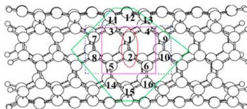
**Figure 76.** ONIOM2 partitioning schemes typically used for investigating atomic functionalization of carbon nanotubes:  $C_2$  high level (red),  $C_{10}$  high level (blue), and  $C_{20}$  high level (green). Reprinted with permission from ref 486. Copyright 2004 Elsevier B.V.
